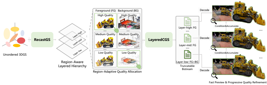
Fig. 1: Object-level scalable compression for 3DGS. Given an unordered 3DGS model, it is reorganized into a region-aware layered hierarchy for region-adaptive quality allocation using RecastGS. The layered feed-forward compressor LayeredCGS then generates a truncatable bitstream for fast preview and progressive quality refinement. Each quality level corresponds to a submodel of cumulative layers, and each layer is encoded as an independent bitstream segment.
